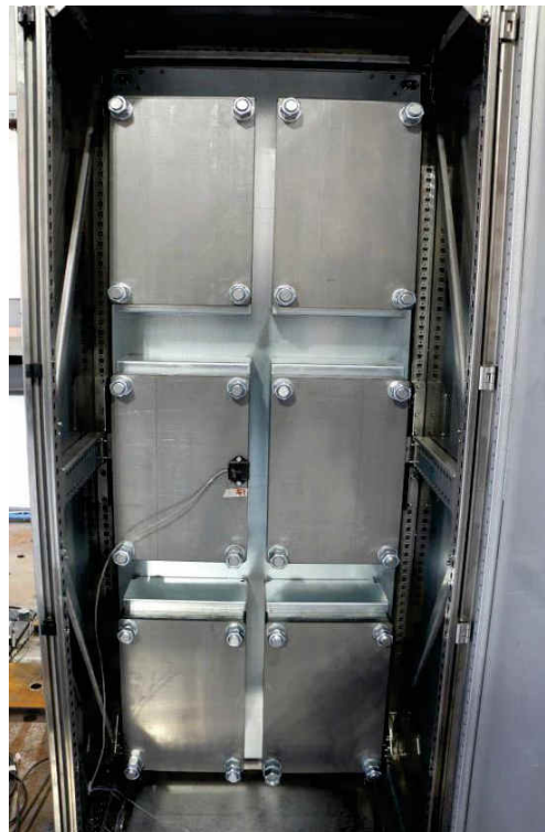
Detail of Weights mounted on internal plate
