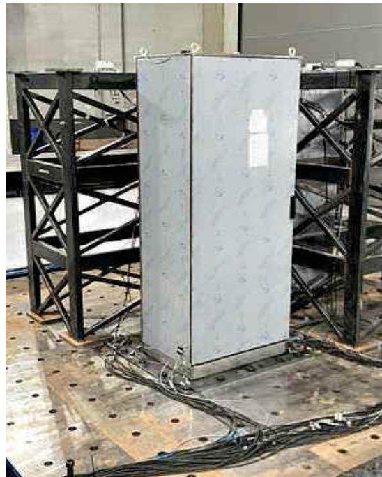
Test Specimen mounted on shake platform
