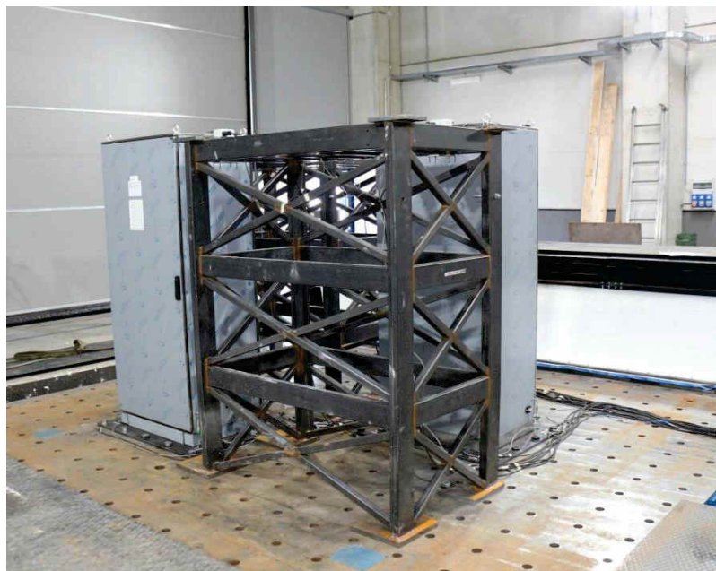
Test Specimen mounted on shake platform
