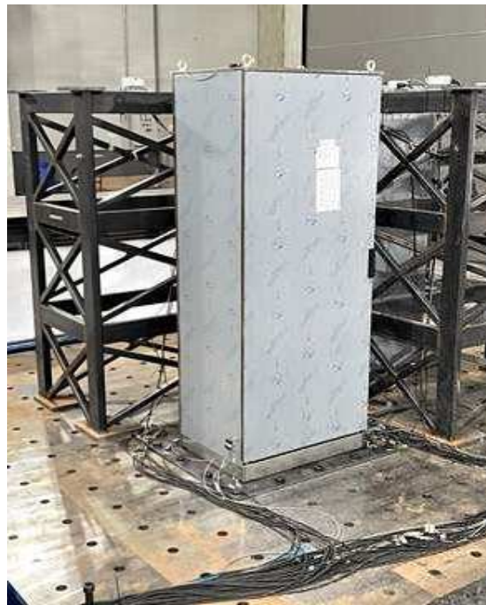
Test Specimen mounted on shake platform
